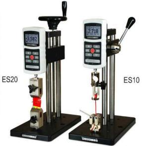
The ES20 is shown in a peel testing application with Series 5 digital force gauge, and film & paper grips.
