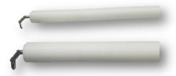
The Children's Finger Probes come in a set of two. One size is for simulation zero to thirty six month old children, Model JFP32A; the second size is for three to fourteen years old, Model JFP32B. These test fingers are to test for protection against access to hazardous parts with a human finger. The jointed finger tips are all made with high quality stainless steel. The handles are fabricated from durable Delrin material.
