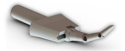
The UL Plastic Articulated Probe is a standard articulated finger as required by Underwriters Laboratories in many of their standards. It is a jointed test probe specifically designed to test equipment likely to be accessible by children.
