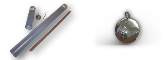
The Impact Tester, Model ITB15A, has been developed in accordance with product safety standards IEC 60065, IEC 60601, IEC 61010, IEC 61032, and IEC 60950. It can be used for many other applications as well. It is used to determine the effectiveness of insulating enclosures and barriers and anywhere the robustness of mechanical assemblies is important. The Impact Test Ball ITB15 is made of chrome plated steel, providing durability and corrosion resistance.
