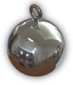
The **Impact Test Ball** is a specially machined ball to test impact resistance according to IEC, CSA and UL Standards. It is made of chrome-plated steel for durability, and is fitted with an eyelet to facilitate testing for pendulum applications. This is called out in IEC 60950, 61032, UL 1989, UL 1418, plus others.
