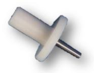
This is a precision probe made in accordance with all IEC standards listed below. The **Test Pin Probe** is used to test for accessibility of small objects and meets IEC, CSA and UL requirements. The probe is made of stainless steel with a Delrin® handle. The stainless steel pin is 3 mm in diameter at the tip. It is tapered over a 15 mm length to finish at 4 mm in diameter at the handle.
