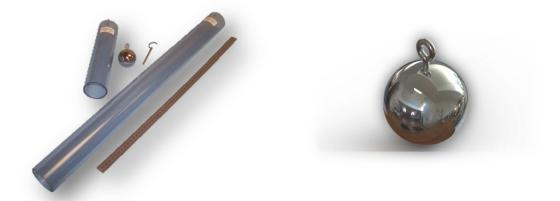
The Impact Tester, Model ITB2A, has been developed in accordance with product safety standards IEC 60065 and IEC60950 and can be used for many other applications. It is used to determine the effectiveness of insulating enclosures and barriers and anywhere the robustness of mechanical assemblies is important. The Impact Test Ball ITB2 is made of chrome plated steel, providing durability and corrosion resistance.
