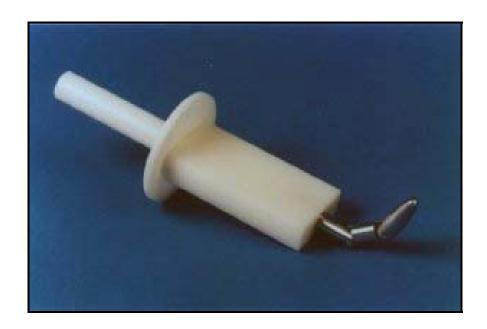
This is a precision probe made in accordance with all IEC standards. Examples are IEC 61032, 60950, 61010 and 60601; and it is also used for Canadian and USA standards. It features a palm simulator and a restricted joint movement, which simulates the characteristics of the human hand. The finger is made of stainless steel and the rest of the instrument is Delrin®. Handle is designed to accept either a banana jack or a force gauge.
