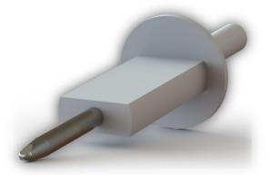
This is a precision probe made in accordance with all IEC standards listed below. It is also used for CSA and UL requirements. The Unjointed Finger Probe is made for forceful insertion where the flexibility of the Jointed Finger Probe would be difficult. The finger is made of stainless steel and the rest of the instrument is Delrin®. The handle is designed with a threaded hole for use with force gauges. The handle also is electrically connected to the fingertip for continuity measurements.
