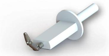
This is a precision probe made in accordance with all IEC standards listed on page two. It is also used for Canadian and USA standards. It features a palm simulator and a restricted joint movement, which simulates the characteristics of the human hand. The finger is made of stainless steel and the rest of the instrument is Delrin<sup>®</sup>. Handle is designed to accept either a banana jack or a force gauge.
