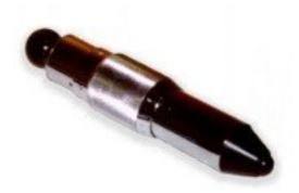
The **Universal Impact Hammer** is designed to perform impact tests for product durability. The UIH20 meets the testing needs of industry standards such as IEC 60065, 60335, 60598, 60601, 61010 and others. The hammer simulates mechanical impact to electronic products and electrical appliances.
