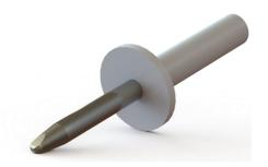
This is a precision probe made in accordance with all IEC standards listed below. It is also used for Canadian and USA standards. The Unjointed Finger Probe is made for forceful insertion where the flexibility of the Jointed Finger Probe would be difficult. The finger is made of stainless steel and the rest of the instrument is Delrin®. The handle is designed with a threaded hole for use with force gauges. The handle also is electrically connected to the fingertip for continuity measurements.
