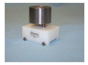
The Scratch Tester, Model ST10, has been developed in accordance with product safety standards IEC60950 and IEC60065. It is used to determine the effectiveness of insulating coatings on printed wiring boards and anywhere the robustness of coatings is important.
