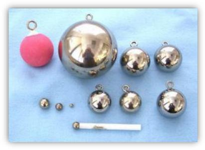
The Impact Test Ball is a specially machined ball to test impact resistance according to IEC, CSA and UL Standards. It is made of chrome-plated-steel for durability, and is fitted with an eyelet to facilitate testing for pendulum and/or vertical drop applications. Eyelet is threaded to the ball to allow attachment of a handle or force gauge. Weights are closely controlled. Other impact test balls are made without the eye, with a handle and/or made of rubber.
