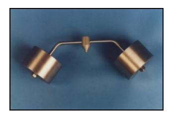
The **Ball Pressure Apparatus** is used to check the integrity of dielectric materials by exerting 20N force. The BPA10 is called out in IEC 60335, 60950, 61010, UL, CSA and European Norms. It is used to check the integrity of dielectric materials by exerting 20N force. The Ball Pressure Apparatus is made of stainless steel for long life. Since accelerated life procedures are used for this oven test, more than one apparatus may be useful for parallel testing.
