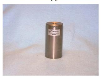
The **Base for the Ball Pressure Apparatus Figure A)** supports the Ball Pressure Apparatus (Figure B) during testing. It is made of stainless steel, with a 2mm hole for thermocouple applications. The base complies with all standards requiring the use of a ball pressure apparatus.
